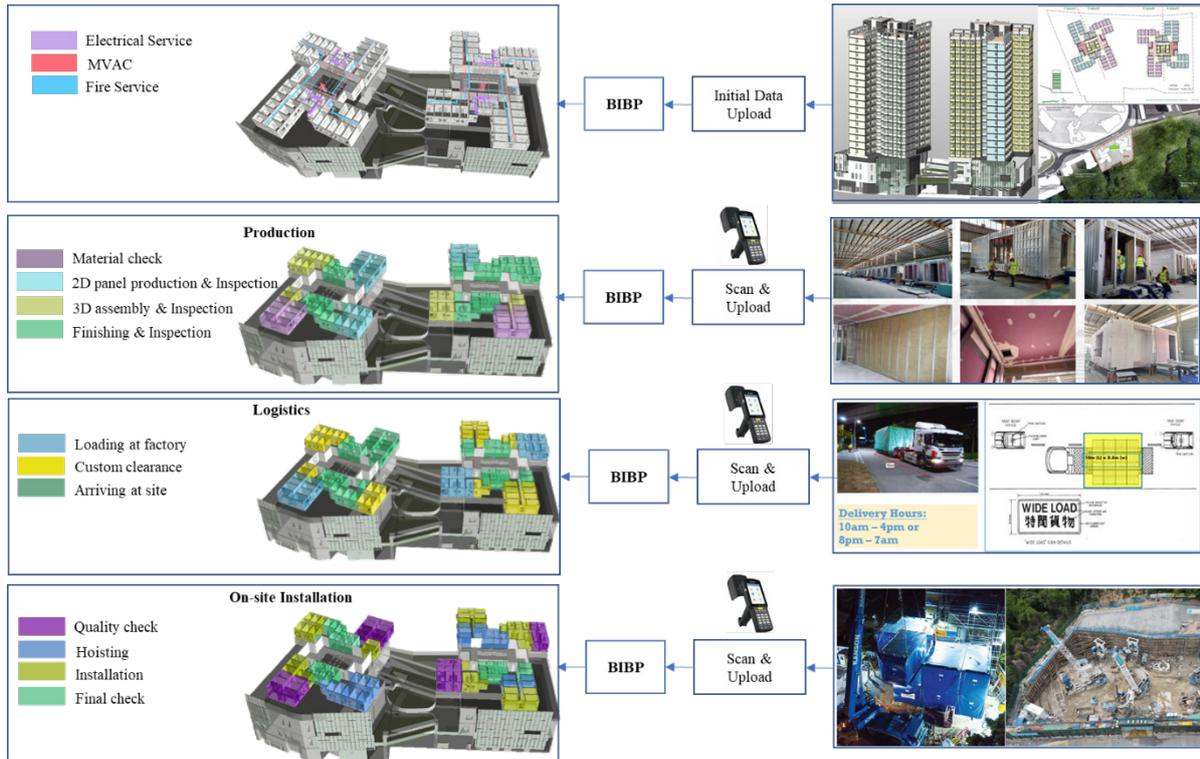
Figure 9. SCM process in BIBP for modular construction
