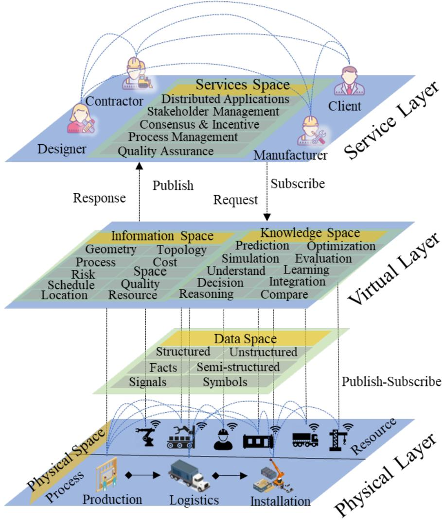
Figure 2. Three-layer DIK-oriented SCM model in modular construction
