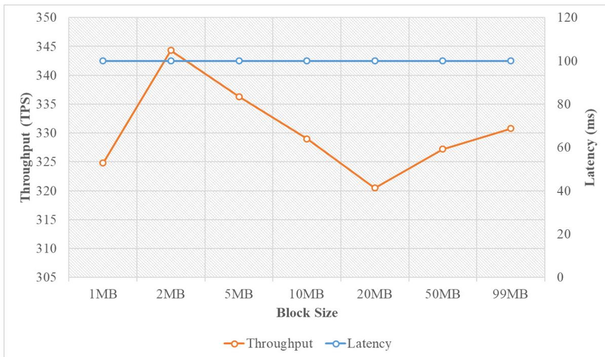
Figure 13. Throughput and latency of the prototype system
