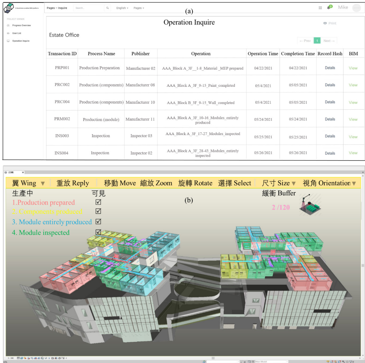
Figure 8. BIBP user interfaces: (a) project client's interface for inquiring about past transactions; (b) function for production progress visualization
